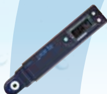
B-111 (Pen type) The pen type sensor allows small samples to be tested.
